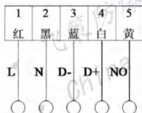
接线箱X端子排 Terminal box X terminal block
